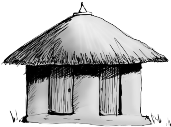
Figure 39: Mud plastered wooden wall/thatched roof
